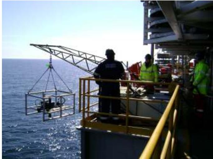
Film-Ocean Lars (LAunch and Recovery System) deploying FRS Marine Laboratory baited camera frame fitted with a Kongsberg digital stills camera and a Nortek Aquadopp from the South side of the QU deck at Nexen operated Buzzard Platform.
