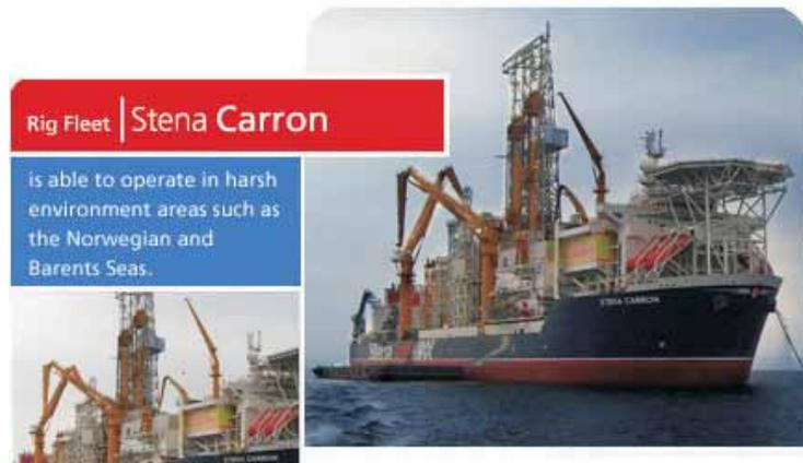
Above: The Stena Carron is a dual-mast, ultra-deepwater, dynamically-positioned drillship, capable of drilling in water depths of up to 10,000ft and has a total drilling depth of up to 35,000ft. This technologically advanced drilling rig is designed to offer maximum safety and operational efficiency in mild and harsh environments, faster transit speed between locations and greater deck load, to accommodate more equipment.
