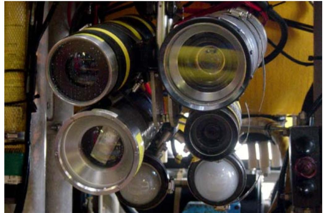
*Kongsberg camera system on the pan and tilt arm. The camera housing is top right, and the flash tube is bottom left. Also mounted on the arm are colour video camera (top left), a low light video (bottom right) and a pair of video lights (right at the bottom),*
