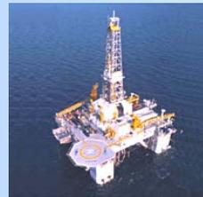
The Jack Bates, A Transocean Semi-Submersible rig, capable of drilling in 1500m of water to a drill depth of nearly 10,000m.
